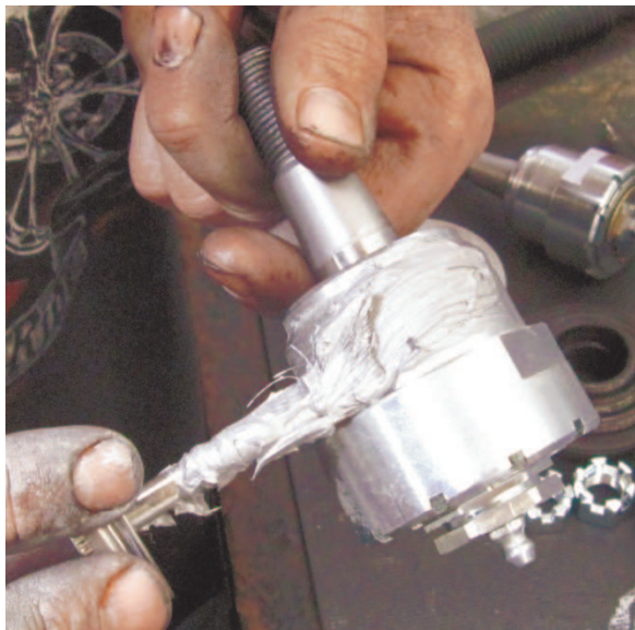
Figure 4, Applying Anti-Seize to ProSteer Body
