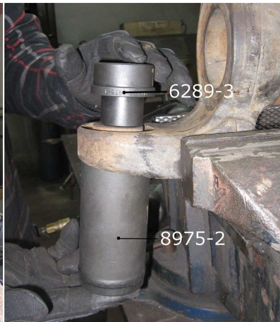
Figure 3, Pressing out OEM Lower Ball Joint
